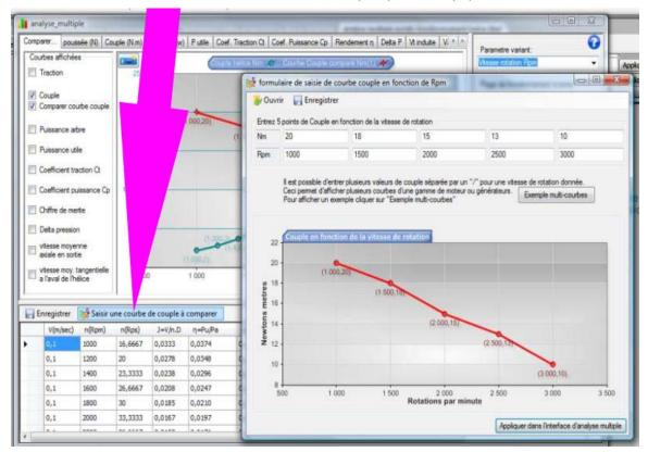
It is possible to enter multiple torque curves representing several motors or generators (3 motors curves in the example below) and editing performance curves, depending on the rotational speed, to view directly the speed of rotation and the performance of the same propeller mounted on a variety of motors or generators of different powers:
